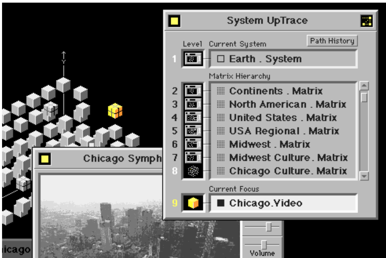
Figure 9: System Up-Trace Panel The system uptrace panel displays fields areas of information. The top field lists the current system , the middle field lists the hierarchy of matrices from highest level down to the lowest currently open, and the bottom field lists the current focus . The user can go instantly to any one of these listed elements or levels by activating the icon (the miniature representation of a screen , matrix , or block ) to the left of the desired destination. The user may also choose to access the Path History function by hitting the Path History button near the top of the system uptrace panel just below the header panel .
